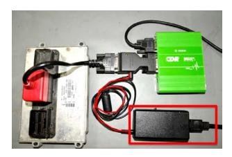
There are two methods, read out the ACM in mounted position also. The ACM can be directly supplied with power when the connection no longer works at the OBD connector. Both methods can cause problems, so it is better, to dismount the ACM and read at a desk or a workbench. An additional advantage occures if the ACM can be kept if possible, since data protection and traceability is ensured (evidence by forensic chain).
